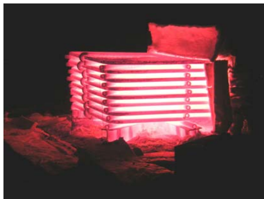
Solution Annealing of the Lower Pendant Loops
